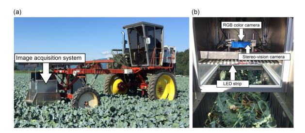
**FIGURE 2** (a) Overview of the image acquisition system that was attached to the prototype robot to acquire broccoli images in the United States. (b) The U.S. image acquisition system consisted of one RGB color camera, one stereo-vision camera, and 21 LED strips for artificial illumination. LED, light-emitting diode. RGB, red-green-blue [Color figure can be viewed at wileyonlinelibrary.com]
