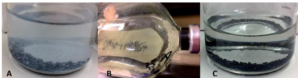
**Figure S1.** Precipitates visualized in the batch bottle of the biotic experiments at day 4(A), and day 14 (B) and bottle of abiotic experiment at day 16 (C) at 70 °C with 9 gL<sup>-1</sup> GAC, 500 mgL<sup>-1</sup> As(III) and Fe(II) respectively.
