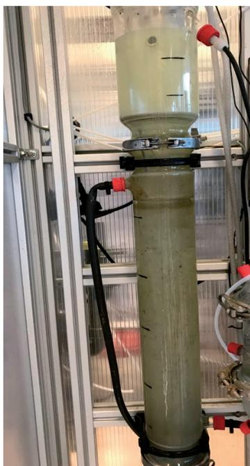
**Figure S3.** Picture of the airlift reactor at day 85. Light green solution typical for scorodite precipitation systems.
