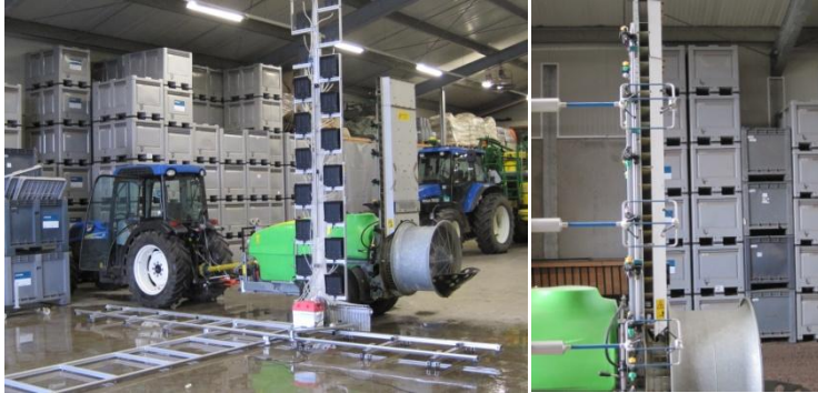
Figure 1. 3-D liquid distribution setup (left) and air-flow distribution setup (right).
