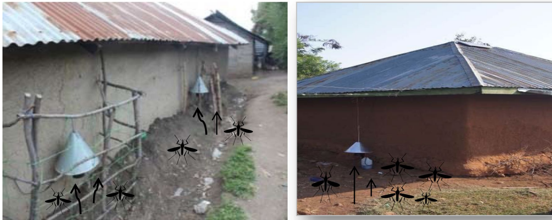
Fig. 1 Placement of solar-powered odor-baited traps for removal trapping of host-seeking mosquito vectors on Rusinga Island in Lake Victoria, western Kenya (Homan et al. 2016). The solar-powered traps were baited with synthetic odor blend and placed outdoors to
