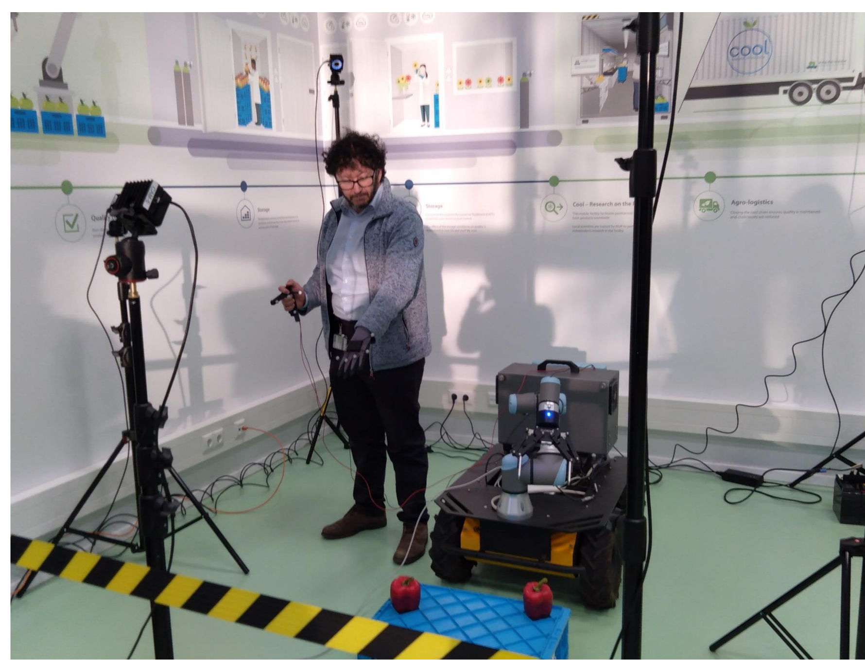
Figure 2. Demonstration of robot teleoperation for picking sweet pepper.
