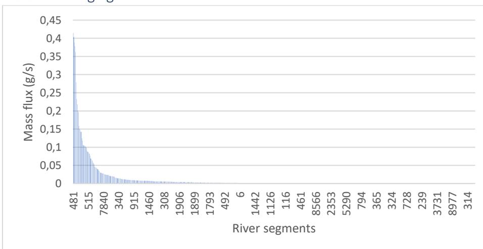
Figure 3 Microplastic flow from cleaning agents
