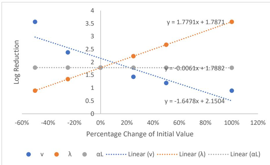
Figure 4.8 Sensitivity analysis of model parameters for a 3m pit latrine
