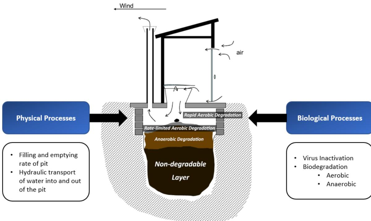
Figure 2.1 Diagram of the processes occurring in pit latrines and its different theoretical layers
