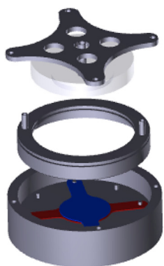
Scheme 1. Flow cell for capacitive separation experiments.
