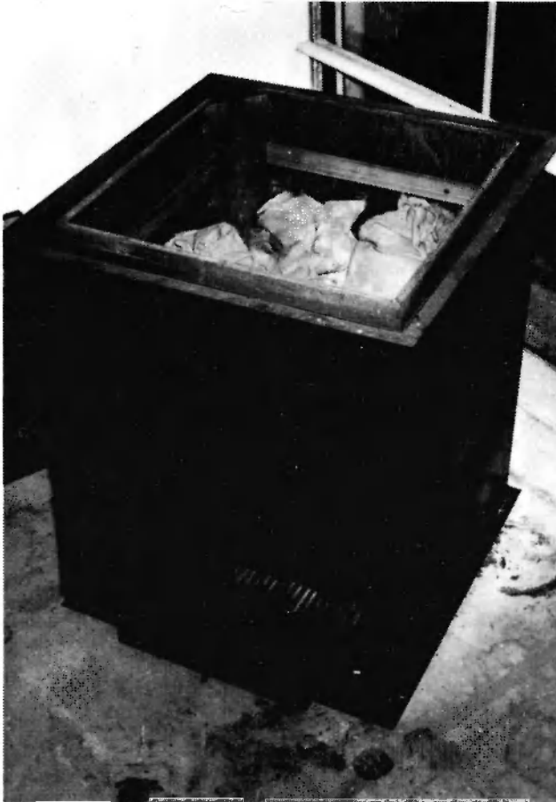
Fig.2 Apparatus for steam sterilisation of soil placed directly above boiling water (inside view).
