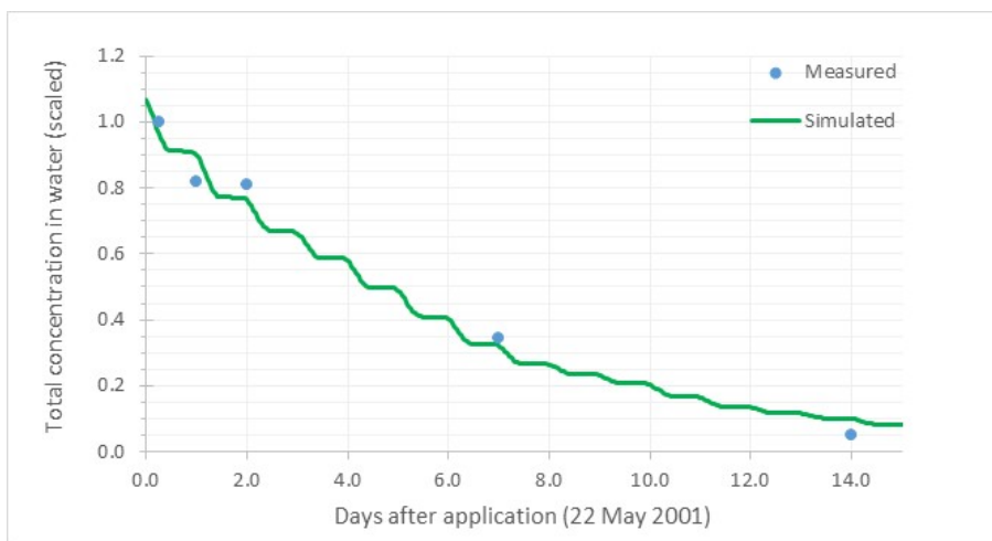
Figure A.4.1 Simulated and measured total concentration (dissolved+ sorbed to suspended solids, \mu\text{g.L}^{-1} ) metribuzin in water as a function of time (d) in the cosm of Fairchild and Sappington (2002). Simulated concentration profile obtained by PEST_TOXSWA optimisation for an initial \text{Deg}T_{50,\text{photo},\text{ref}} = 5 d and an initial loading of 1000 \text{ mg m}^{-2} .
