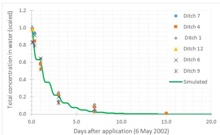
Figure A.4.3 Simulated and measured total concentration (dissolved+ sorbed to suspended solids, \mu\text{g.L}^{-1} ) metribuzin in water as a function of time (d) in the ditches of Arts et al. (2006). Simulated concentration profile obtained by PEST_TOXSWA optimisation for an initial \text{DegT}_{50,\text{photo},\text{ref}} = 1 d and an initial loading of 500 \text{ mg m}^{-2} .
