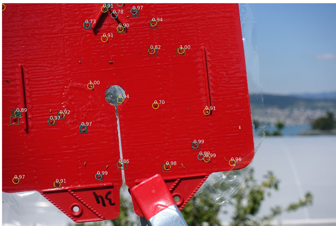
Figure 4. Detection of female spotted wing drosophila (SWD) (yellow) and male SWD (blue) in an image of a manually prepared sticky trap that was placed on a static position outside in the field. The image was taken by a camera carried by a flying UAV. Rectangles indicate the ground truth and circles indicate the model predictions. White numbers are the confidence levels of the predictions.
