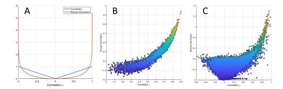
**Figure 8.** (A) MI  $MI(X_1, X_2)$  of two bivariate variables  $X_1$ ,  $X_2$  linearly correlated with correlation  $\rho$  as a function of  $\rho$ . The two curves intersect at approximately  $\rho = 0.916$ . (B) MI versus Pearson's correlation from data simulated with an average correlation of 0.6 (beta simulation). (C) MI versus Pearson's correlation from experimental data (data set 3 from Table 1).
