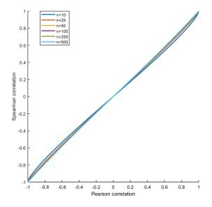
**Figure 10.** Relationship (see Equation (5)) between the Spearman's (Equation (7)) and the Pearson's (Equation (6)) correlation coefficients for linearly correlated data for different sample size *n*.
