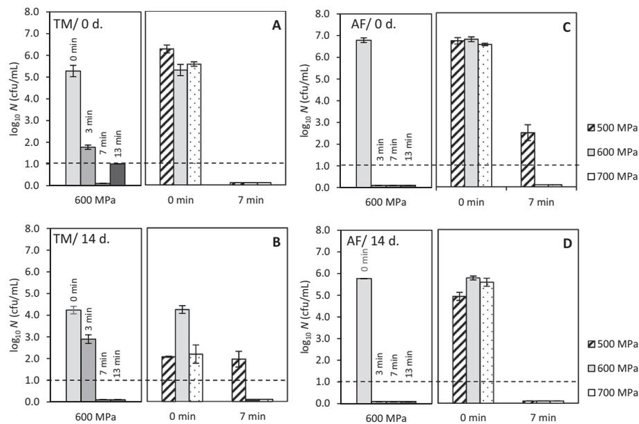
**Fig. 6.** Viable counts of *Talaromyces macrosporus* (TM) (A + B) and *Aspergillus fischeri* (AF)(C + D) suspended in strawberry puree that received a pre-heating step of 2 min followed by high pressure treatment at indicated pressure and holding time at a maximum temperature of 90 °C. A + C) directly plated at t = 0 days, or B + D) plated after 14 days storage at 25 °C. Dashed line indicates the detection limit.
