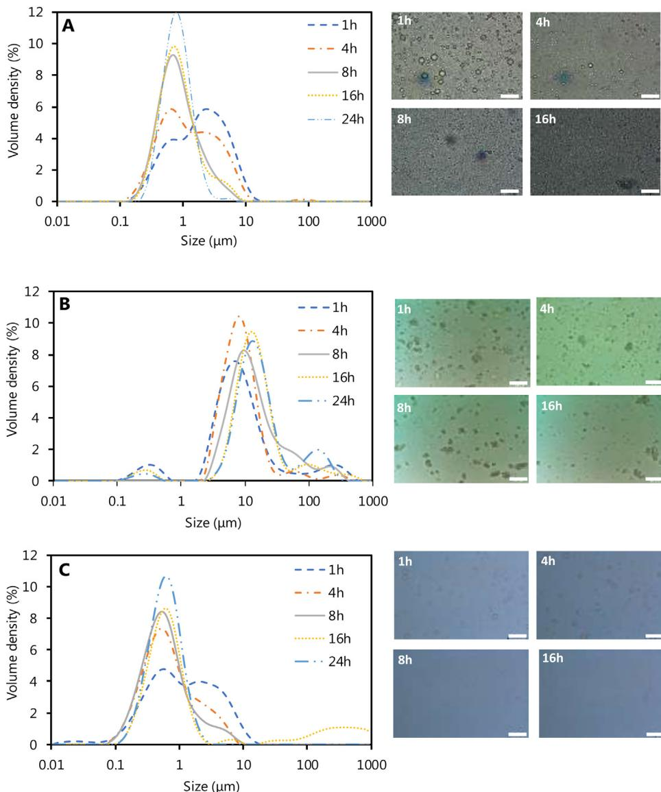
**Fig. 4 – Particle size distribution and micrograph of oleosome diluted creams recovered at (A) pH 9.5 with NaHCO<sub>3</sub> 0.1 mol/L, (B) at pH 7 with H<sub>2</sub>O and (C) at pH 7 with H<sub>2</sub>O and 1 wt. % SDS. Scale bar 20 μm.**
