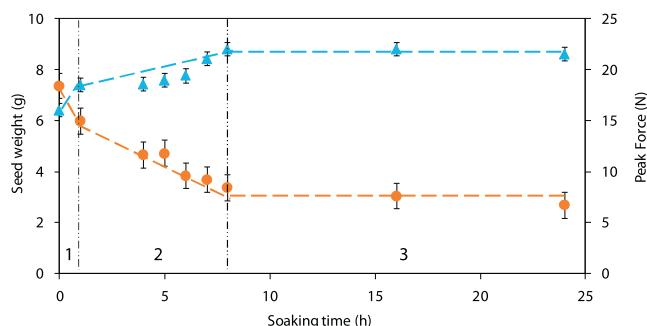
**Fig. 1 – Effect of soaking time on the rapeseed weight (g) (▲) and peak force (N) (●) or necessary force to break a rapeseed. Three different stages of water absorption and modifications on the strength of the material are observed. (1) A steep increase on water content and loss of strength. (2) A less steep increase of water content and loss of strength (3) A plateau region with no variation in seed weight or seed mechanical properties.**
