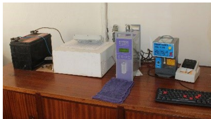
Picture 1. Milk analyser and accessories used in Mbarara for determining the milk quality for the QBMPS. Photo taken by Asaah Ndambi
