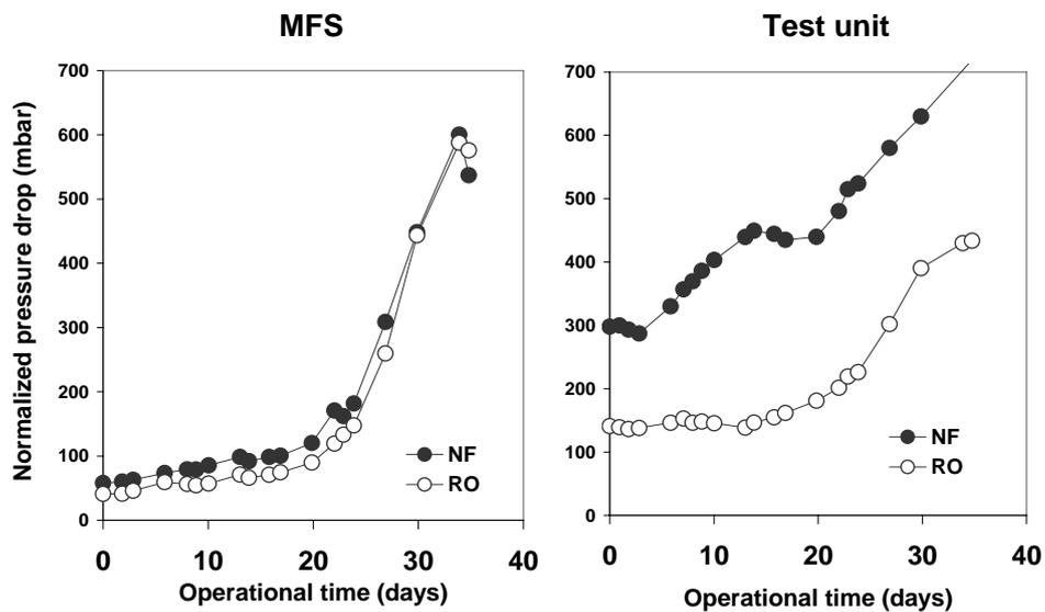
Fig. 6.2 Normalized pressure drop increase in the MFS system and in the membrane test unit (bench scale) supplied with feed water of the RO installation at location 2.
