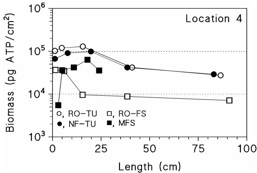
Fig. 7.6. Biomass concentrations in the membrane elements of the test unit at location 4. RO-TU: RO membrane of test unit; NF-TU, NF membrane of experimental test unit. RO-FS: membrane from full scale plant; MFS, membrane fouling simulator.
