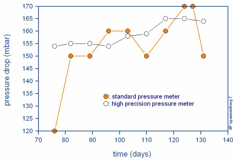
Fig. 5.3 Pressure drop in membrane element at location 1, as determined with a standard procedure and with a pressure difference sensor.
