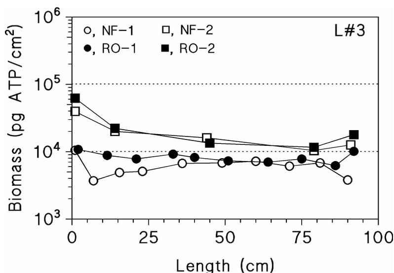
Fig. 7.5. Biomass concentrations in membrane elements at location 3. RO-1: RO membrane from experimental test unit; first experimental period; NF-1, NF membrane from experimental test unit, first experimental period; RO-2, NF-2, second experimental period.
