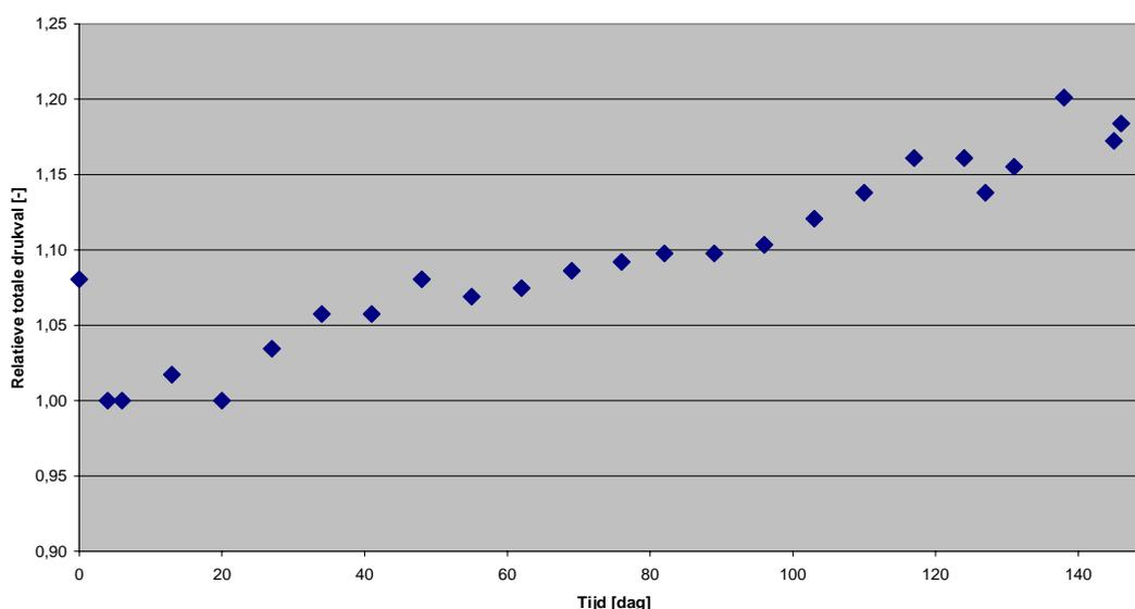
Fig. 6.1 Increase of feed channel pressure drop in the pilot plant membrane installation at location 1.
