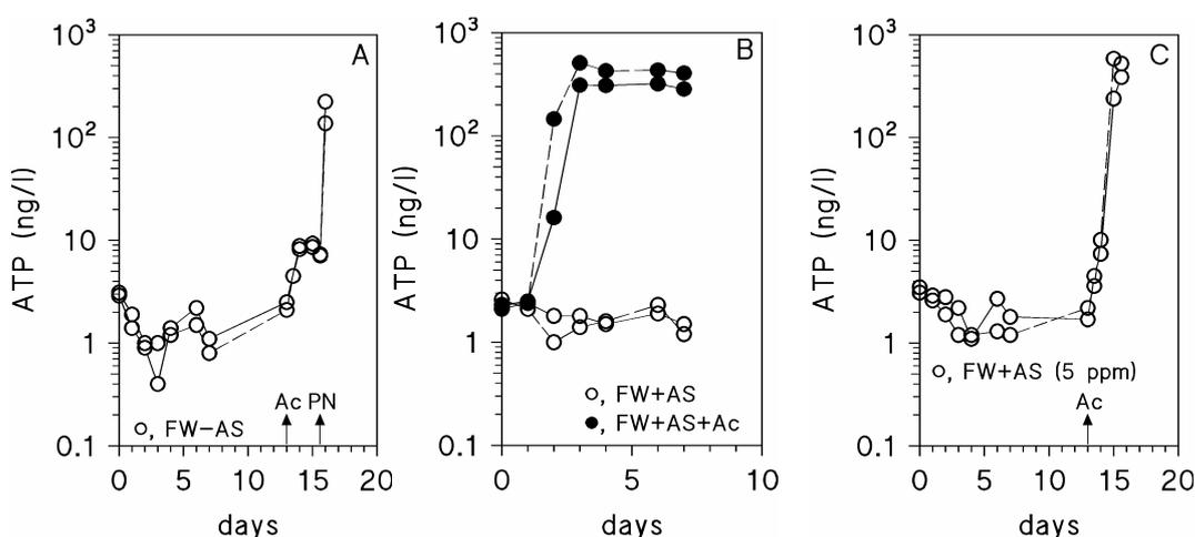
Fig. 1. A, Production of biomass (ATP) in batch tests with water sampled after ultrafiltration and acid dosage, supplemented with acetate (1 mg/l C) on day 13 and P+N on day 15; B, feed water sampled after AS dosage (0.9 mg/l), and supplemented with acetate (1 mg C/l) on day 0; C, Feed water after dosage of acid, supplemented with AS (5 mg/l) and P+N on day 0 and with acetate (1 mg C/l) on day 13.
