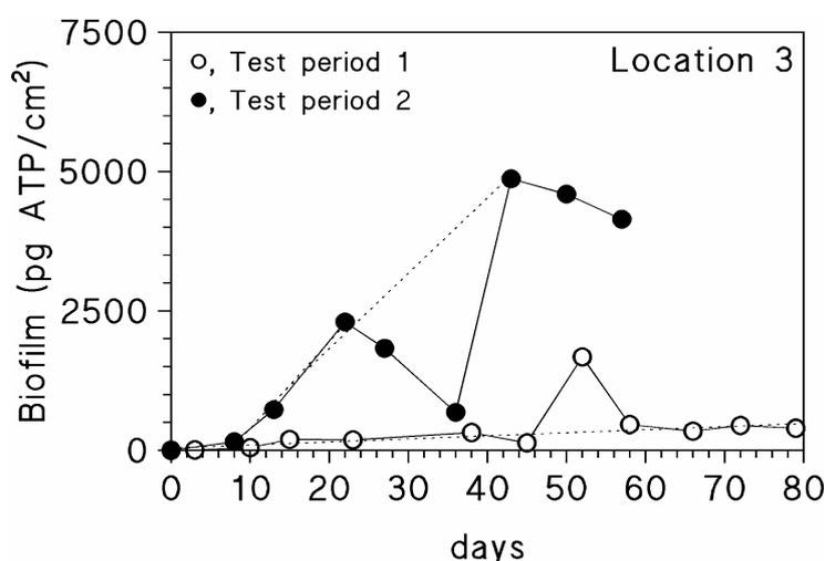
Figure 4.3 Biofilm concentration in the biofilm monitor in two periods of investigation on UF filtrate. .
