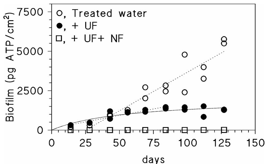
Fig. 4.1 Effect of ultrafiltration (UF) followed by nanofiltration (NF) on the biofilm formation in the biofilm monitor. The treated groundwater contains a high concentration of NOM (NPOC= 8 ppm).
