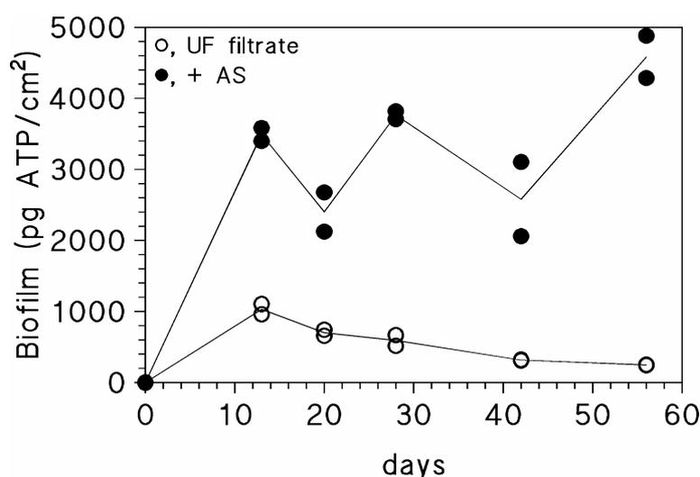
Figure 4.2 Biofilm concentration in the biofilm monitor before and after AS dosage.
