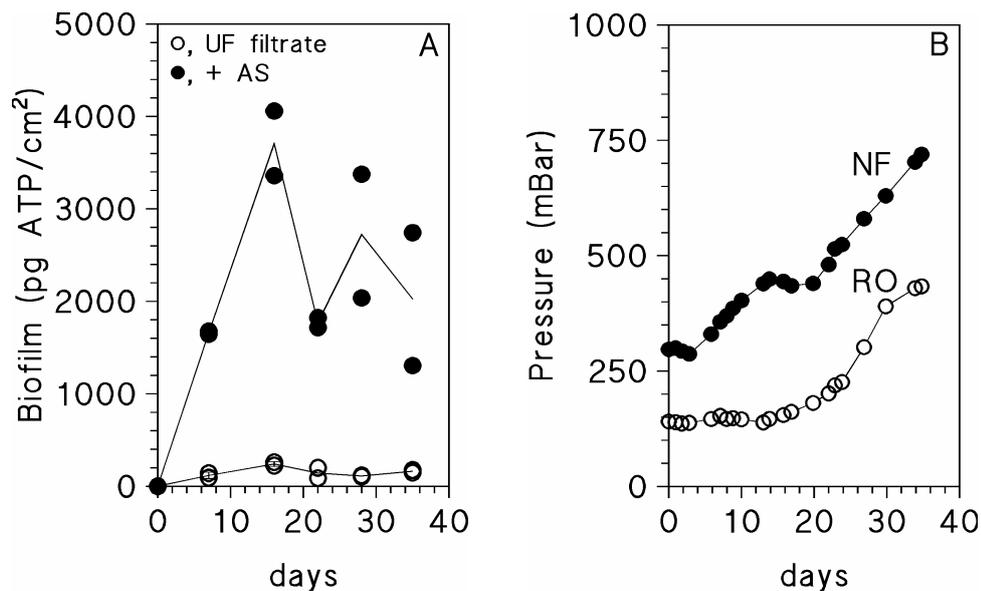
Fig. 2. A Biofilm formation in the biofilm monitor at location B supplied with water from open storage reservoirs, treated by coagulation/sedimentation and ultrafiltration. B. Feed channel pressure drop in bench scale membrane elements (RO and NF, 4") supplied with UF filtrate after AS dosage.
