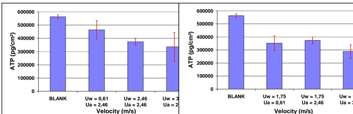
Figure 4: Biomass removal from PVC-P rings measured with ATP using different water flows at a constant air flow of 2.46 m/s (n=4).
