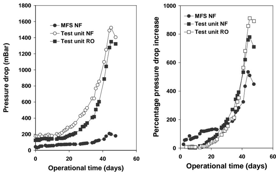
Fig. 6.6 Increase of the feed channel pressure drop in the MFS and in the test unit supplied with feed water at location 4.
