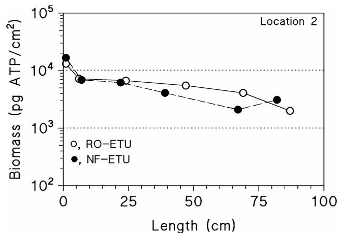
Fig. 7.4. Biomass concentrations in membrane elements at location 2. RO-ETU: RO membrane from experimental test unit; NF-ETU, NF membrane from experimental test unit; FS, full scale plant.
