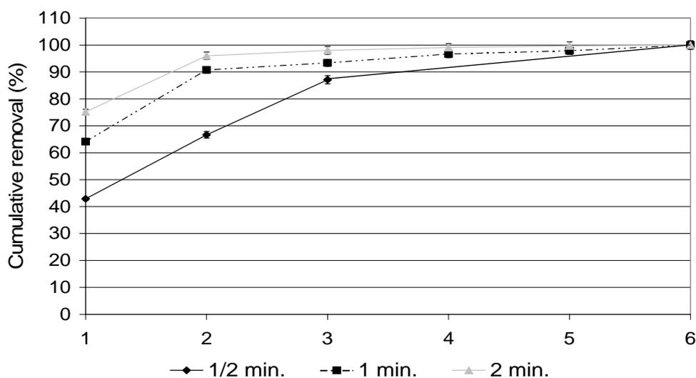
Figure 7.1 Biomass removal from pieces of plasticized PVC using 3xHES during 1/2, 1 and 2 minutes at 45%; 1 to 5 is 1 to 5 times HES; 6 is the swab treatment; 100% is 28926, 18023 and 17812 pg ATP/cm<sup>2</sup>, respectively.
