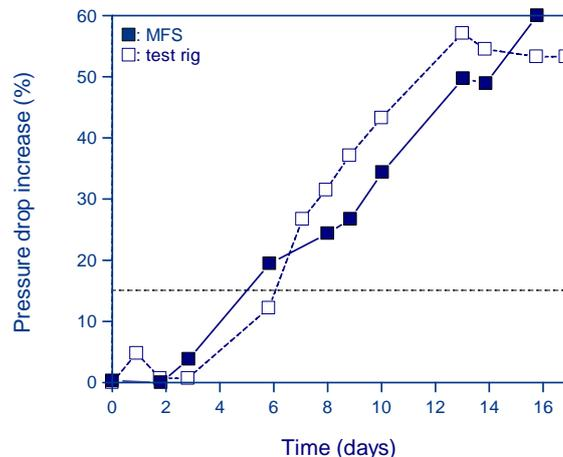
Figure 6.2. Pressure drop increase (% of start value) of the MFS and test unit supplied with the RO feed water including 3 ppm antiscalant.
