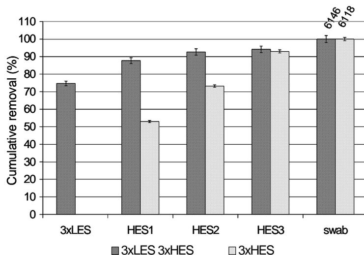
Figure 7.2 Biomass removal from sample pieces of an NF-membrane, using low energy sonication (LES) and/or high energy sonication (HES). The amount obtained after additional swabbing is considered to represent the total amount (100%) of attached biomass.
