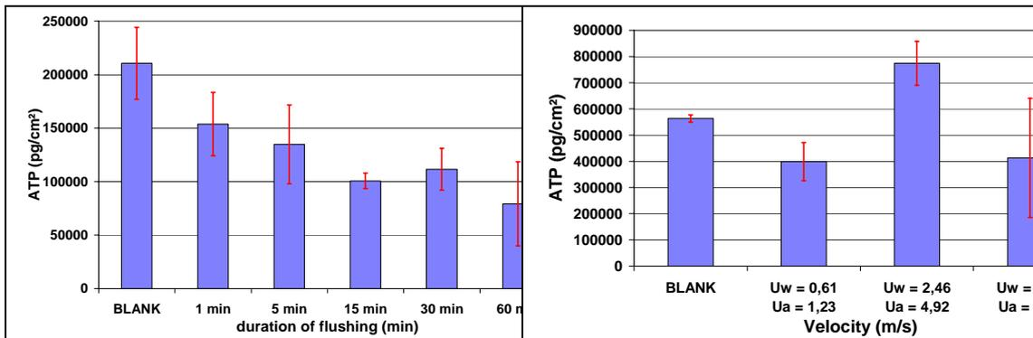
Figure 2: Biomass removal from PVC-P rings measured with ATP using different periods of air-water flushing at a constant air water ratio of 2:1 (n=4).
