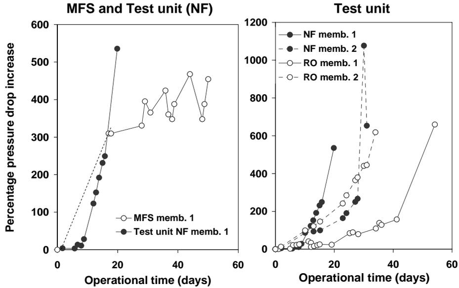
Fig. 6.5 Percentage increase of the feed channel pressure drop in the MFS and in the test unit supplied with water prior to AS dosage in two experimental periods at location 3.
