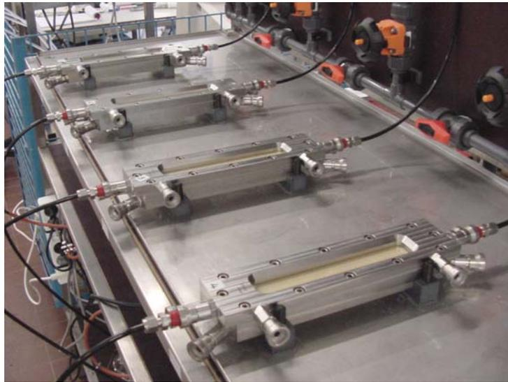
Figure 5.4 Four Membrane Fouling Simulators (MFS) installed in parallel during comparison studies. The external dimensions of a MFS is 0.07 x 0.30 x 0.04 m.
