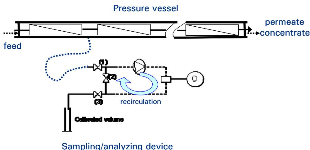
Fig. 5.1 Analyzing device and positioning of the sample points
