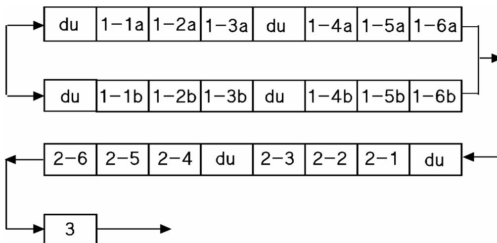
Fig. 3.1 Schematic of the NF pilot plant as used at test location 1. Du = dummy (no membrane element in vessel). Membrane elements 1-1b and 3: no permeate production.
