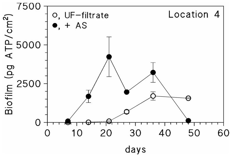
Figure 4.4 Biofilm concentration in the biofilm monitor prior to and after AS dosage at location 4.
