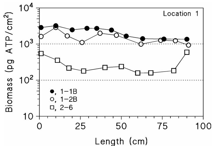
Fig. 7.3. Biomass concentrations in NF elements at location 1. Nrs 1, first element from 1<sup>st</sup> stage; nr 2 element from second stage. Run time: 146 days.
