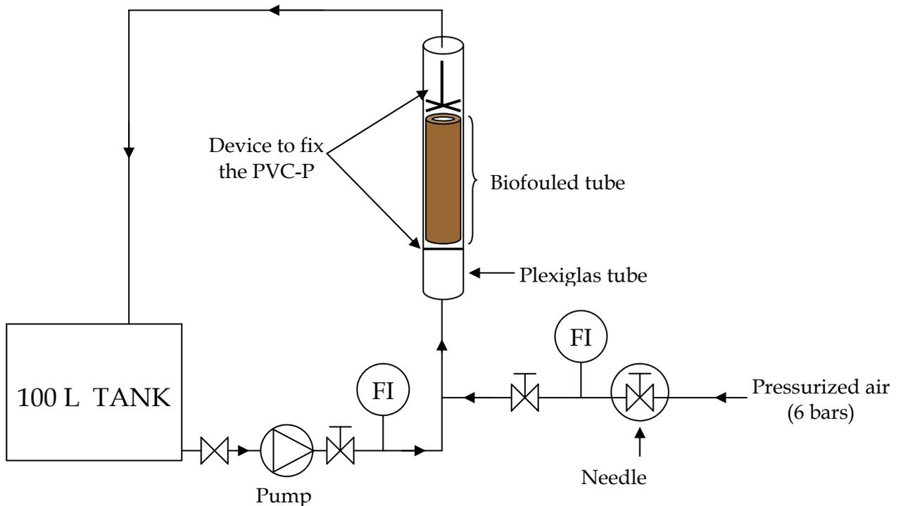
Figure 1: set-up used for assessment of the efficiency of flushing procedures using air/water.
