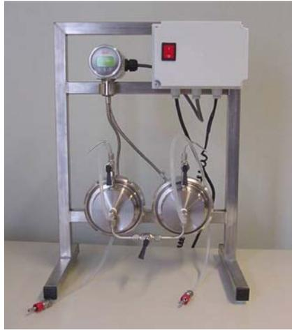
Figure 5.2 Front view of the Differential Pressure Transmitter. Quick connectors are used for assessment of the pressure difference.
