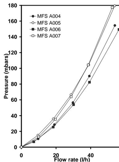
Figure 5.5 Relationship between flow velocity (m/s) and pressure drop (mbar) of 4 MFS's containing different sheets of membrane and spacers.
