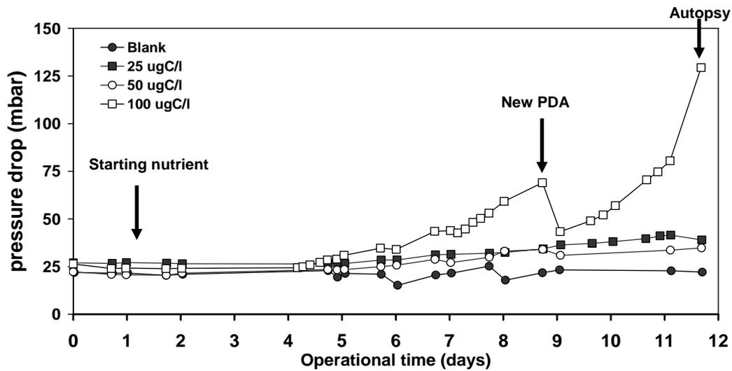
Figure 5.6 Pressure drop increase (%) as function of time with different nutrient concentrations in the feed water of the MFS. New DPA = new pressure drop equipment applied.
