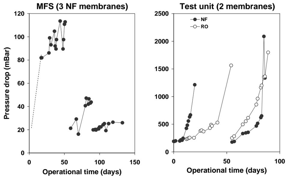
Fig. 6.4. Pressure drop increase in the MFS unit and in the test unit in the two experimental periods at location 3. Feed water: UF product, without AS dosage.
