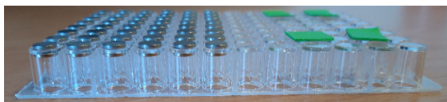
Fig. 2. Magnet plate to pull down the streptavidin beads. Only half of the plate will contain beads, so there is no need for a full plate of magnets.
