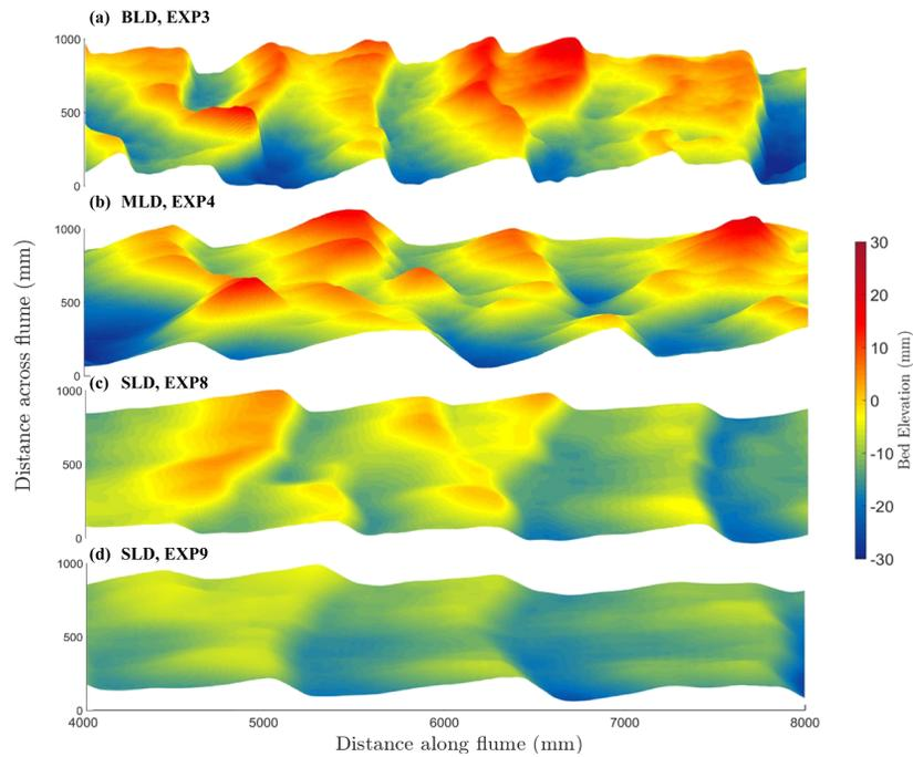
**Figure 2.** Bed morphology under dynamic equilibrium illustrating different stages of dune development and transition to upper stage plane bed, (a) at the bed load dominated (BLD, EXP3), (b) mixed load dominated (MLD, EXP4), and (c and d) suspended load dominated (SLD, EXP8, and EXP9) sediment transport conditions.
