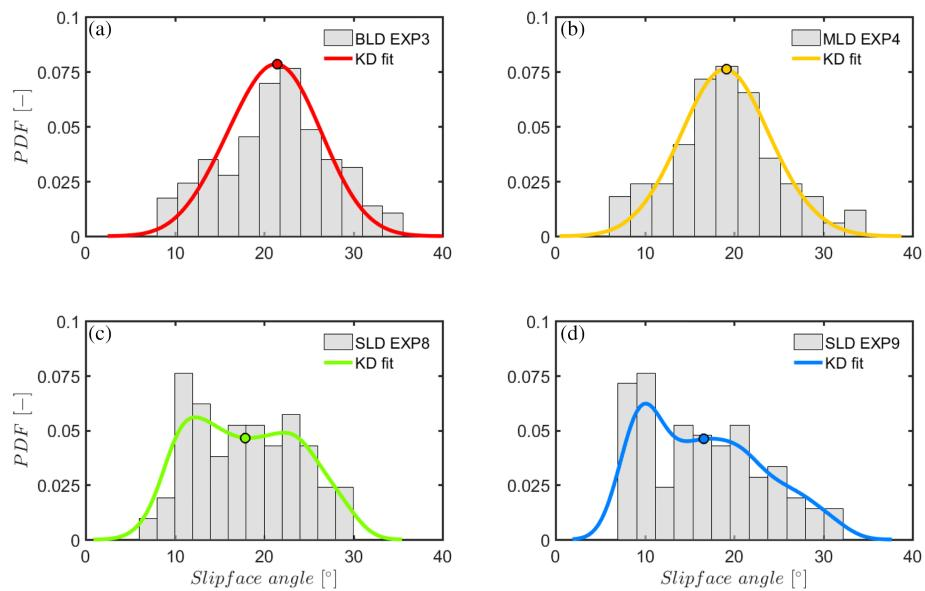
**Figure 4.** Distribution of dune slipface angle for different stages of dune development. The solid lines represent kernel density fits to dune slipface data with circles indicating spatially averaged values, (a) at bed load dominated (BLD, EXP3), (b) mixed load dominated (MLD, EXP4), and (c and d) suspended load dominated (SLD, EXP8, and EXP9) transport conditions.
