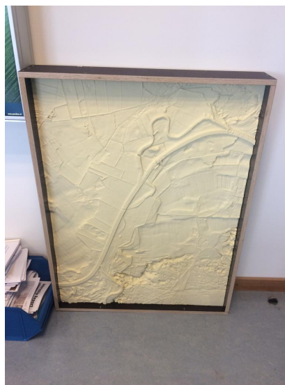
Figure 3: the mold: an inverted DEM of the study area, z-values have been 8 times exaggerated
