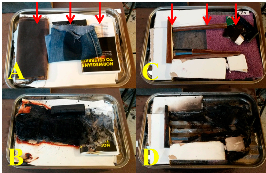
Figure 3. Experimental setup of small scale fires. (A,C) show intact substrates to which 15 mL of white spirit has been applied in three vertical lines (indicated with red arrows) and (B,D) are the corresponding fire debris samples. Substrates for (A,B): vinyl flooring (primary substrate, 60 wt %), plus curtain, wooden chair, magazine, and clothing (secondary substrates, 10 wt % each); substrates for (C,D): plasterboard (60 wt %), carpet material, carpet underlay, floor skirting, and computer fragments (monitor, print boards, and cables) (10 wt % each).
