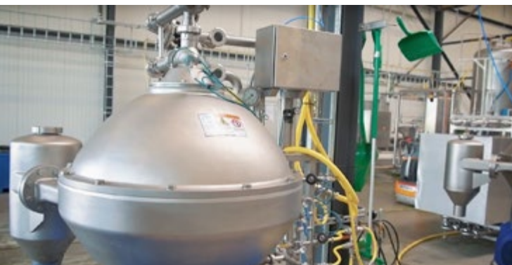
The juice is purified, rid of colour, smell and flavour, and dried into protein powder.
