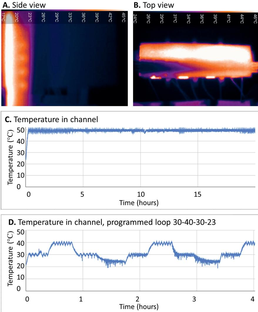
Figure 7.3: Temperature stability within the millifluidics device A) Thermal camera image of the side view of the millifluidics channel. B) Thermal camera image of the top view of the millifluidics channel. C) Temperature in channel as determined with the thermistor at output when the temperature is set at 50°C. D) Channel temperature as determined with the thermistor at output when the temperature regulation is set to a loop of 30 – 40 – 30 – 23°C.
