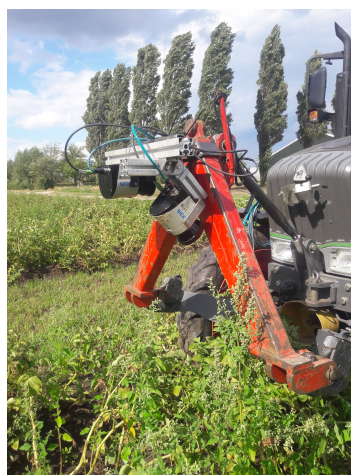
Figure 1. The sensor setup mounted to the tractor's three-point linkage. Here shown while scanning a different crop.
