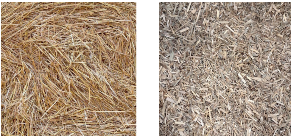
FIGURE 8 REEDS BEFORE (LEFT) AND AFTER GRINDING (RIGHT)
