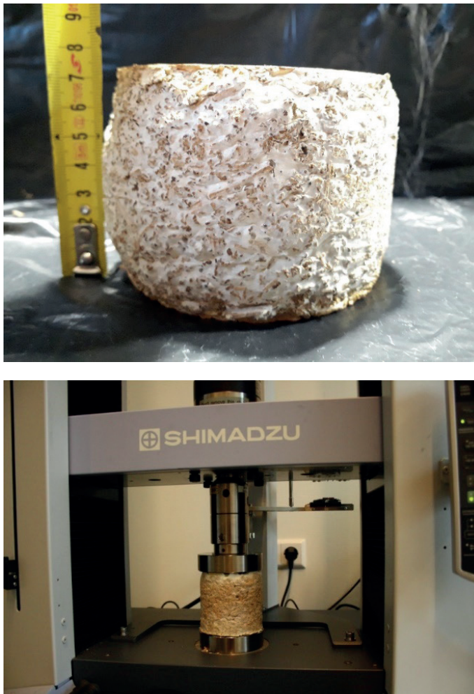
FIGURE 24 DEFORMED HEAT PRESSED SAMPLE (TOP) AND PRESSURE TEST (BOTTOM)
