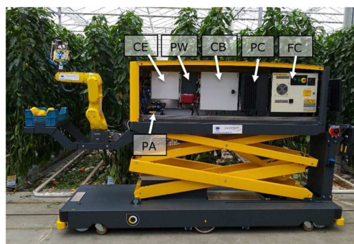
FIGURE 3 The SWEEPER prototype consists of a Fanuc LR Mate 200iD robot arm mounted on an automated cart with a scissor lift. The end effector mounted at the tip of the robot arm contains a cutting mechanism, an imaging system, and a fruit catching device. The photo shows the prototype with the side panel opened. CB, controller box power and network; CE, controller box end effector; FC, FANUC robot controller; PA, compressor for pressured air; PC, computer; PW, power inverter [Color figure can be viewed at wileyonlinelibrary.com ]
