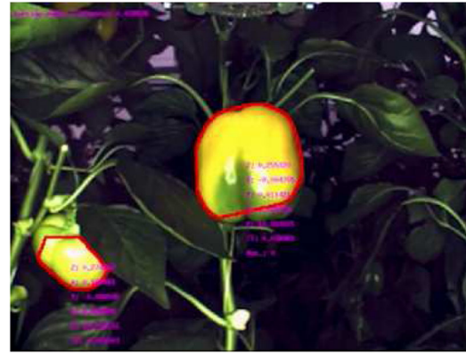
FIGURE 7 Example of real-time fruit detection. The red curves indicate detected areas [Color figure can be viewed at wileyonlinelibrary.com ]
