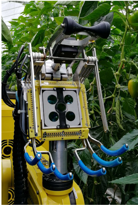
FIGURE 5 End effector with cutting device, Fotonic F80 camera, LED illumination, and fruit catching device [Color figure can be viewed at wileyonlinelibrary.com ]
