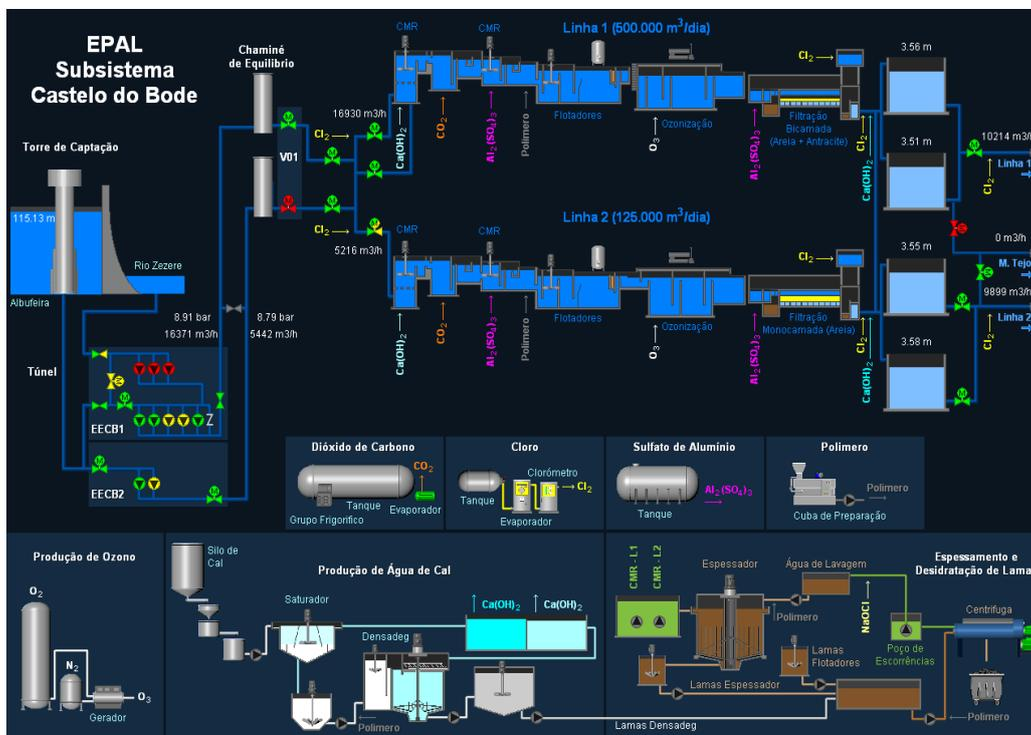
Figure 6.6: Synoptic flow diagram of Asseiceira WTP
