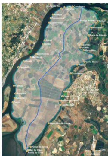
**Figure 6.13: General map of the Lezíria Grande de Vila Franca de Xira PIP. Main drainage channel (blue line) and gates for water intake and drainage – “Portas de Água” (yellow circles). Background image from ESRI basemap. Adapted from ARHT (2009).**
