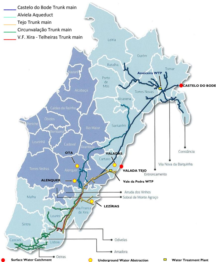
Figure 6.2: EPAL production & transport system and municipalities supplied.
