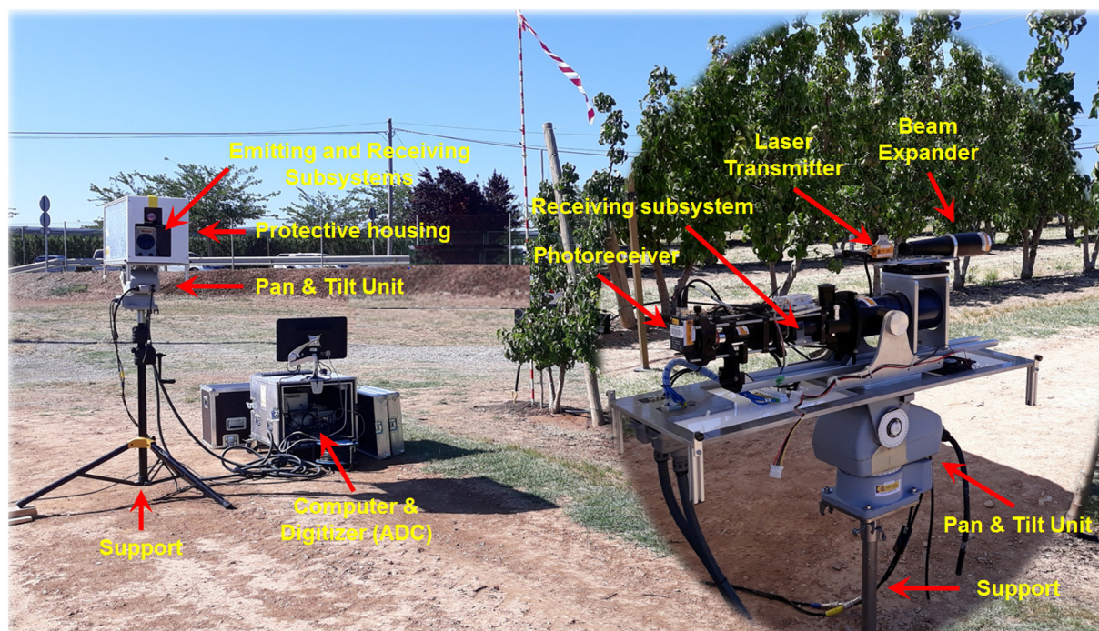
Fig. 2. (Left) LiDAR system used for the spray drift assessment in tests T5, T6 and T7; (Right) zoom view of the emission and receiving subsystems (without the protective housing) where internal optoelectronic components are shown.
