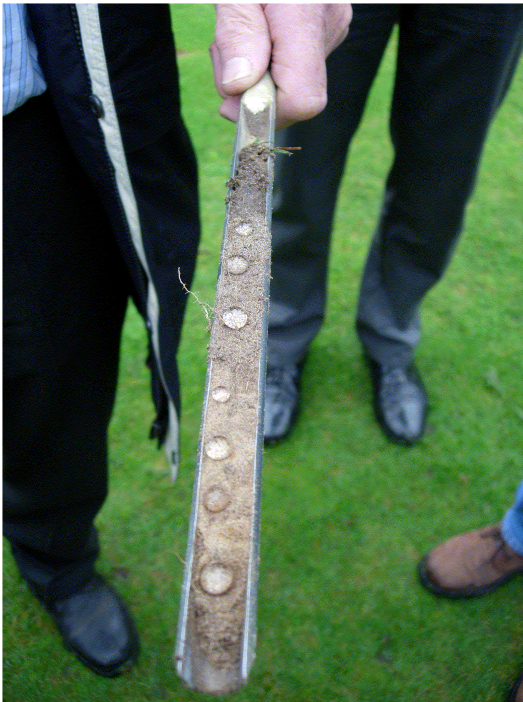
Figure 2.2 Determination of the occurrence, depth and thickness of a water repellent layer in the field, by using a small core sampler.
