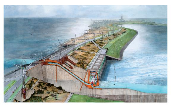
Figure A.6: Dike section of the Valmeer with the pumping system (Illustration by the Das brothers). Source: https://www.deingenieur.nl/artikel/lievense-de-man-van-het-opslagbekken
