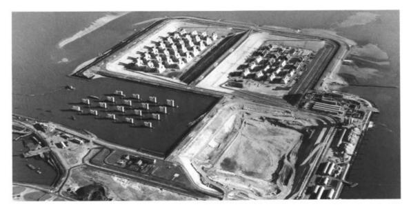
Figure I.4: Eastern Scheldt construction yards. One compartment flooded.
