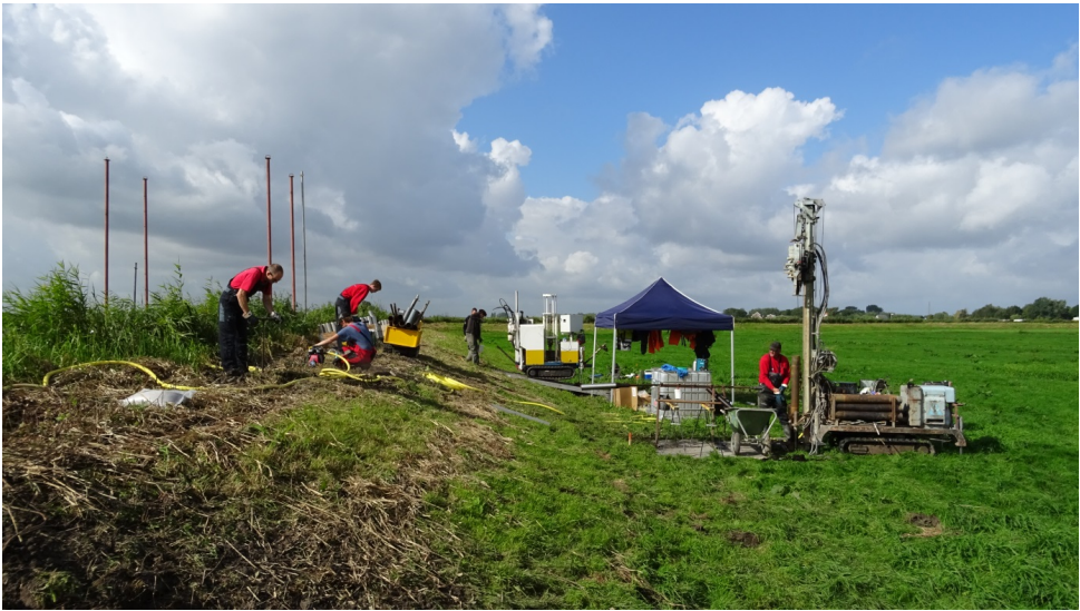
Figure 2.5: Site investigation at location B. Hand borings and installation of standpipes on the crest of the dyke. CPT investigation in progress on the slope and boring/sampling in the polder.
