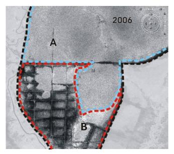
Figure 14. Peat swamp degradation (B) and restoration (A) in the Mawas area between 1998 (JERS-1) (left) and 2006 (PALSAR) (right). The red area is degraded, the blue area is intact or regenerating.
