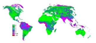
Figure 1. Persistent cloud cover prevents optical remote sensing monitoring of the world's tropical rain forest areas. The colour code shows the estimated number of months per year LANDSAT fails to deliver useful images (Source: [2]).
