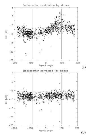
Figure 3. Slope correction for all pixels in a small test area in a mountainous section of central Borneo; (a) backscatter (gamma in dB) as function of slope aspect; (b) idem, after correction (Note: the vertical lines present the radar orientation angles).
