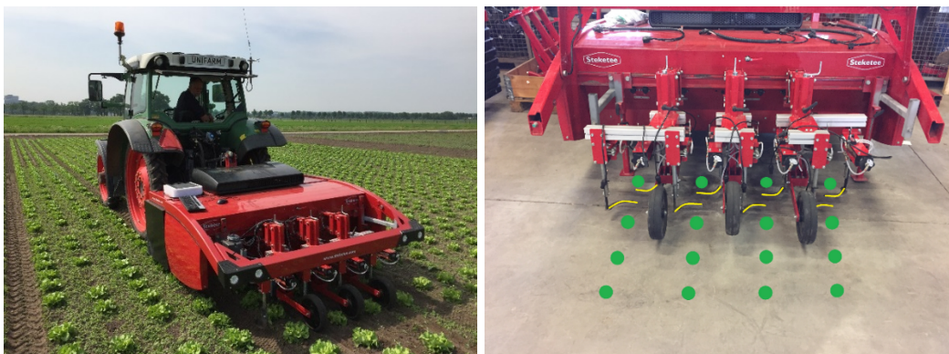
Figure 181. The Steketee IC hoeing machine mounted behind a tractor (left photo) and visualization of the hoeing knives (marked by yellow lines) between the crop plants in the row (marked by green dots) (right photo).
