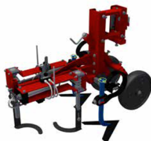
Figure 182. Hoeing actuator of the Steketee IC hoeing machine. The arc shaped knives can rotate to hoe between single crop plants in the row. The V shaped hoeing element is for hoeing between the crop rows.
