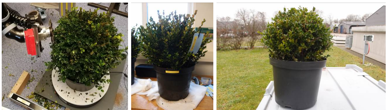
Figure 45. left; end-effector mounted on the manipulator during a lab test. The bush is set on a rotation table to provide access from all sides. Middle; bush before trimming and after trimming; right.
