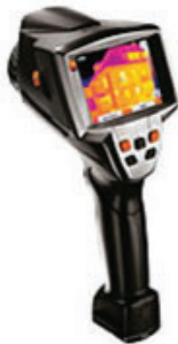
Figure 1: Infrared thermographic camera used to verify the distribution of temperature on piglet skin
