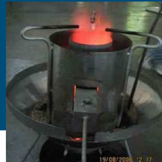
Pictorial of the Continuous-Flow Rice Husk Gasifier
