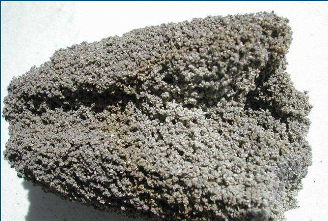
Bed agglomerate removed from a fluidized bed combustor burning a blend of 10% rice straw in wood fuel after 3.5 h of operation.
