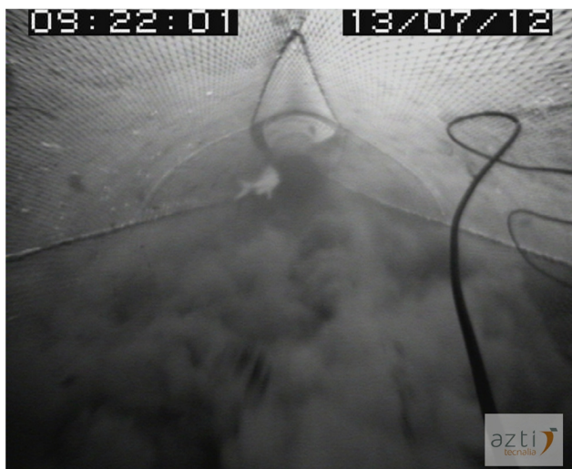
Figure 3.6: Snapshot from an underwater video showing the presence of turbidity in the lower section of the net in the vicinity of the SMP.
