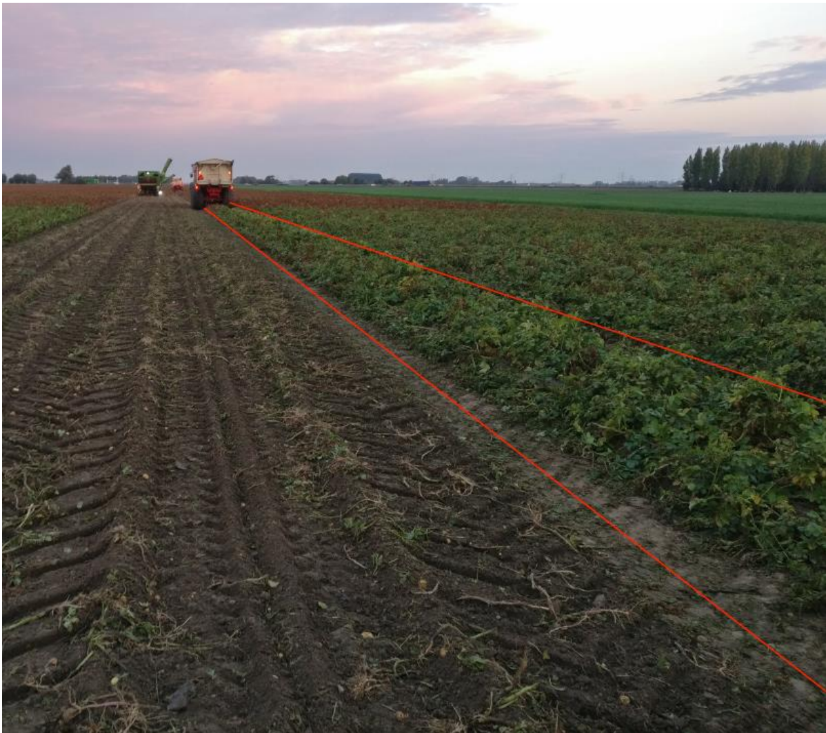
Figure 5: Harvesting operation in which a service unit is traversing an unharvested spray path (red lines) to get to the primary unit. The service unit satisfies both restrictions.
