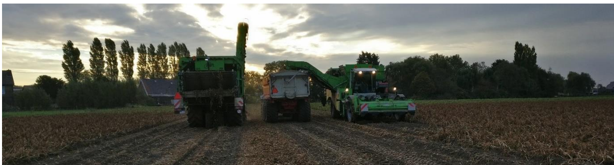
Figure 2: A primary unit (right) unloading onto a service unit (middle) and another primary unit harvesting (left).
