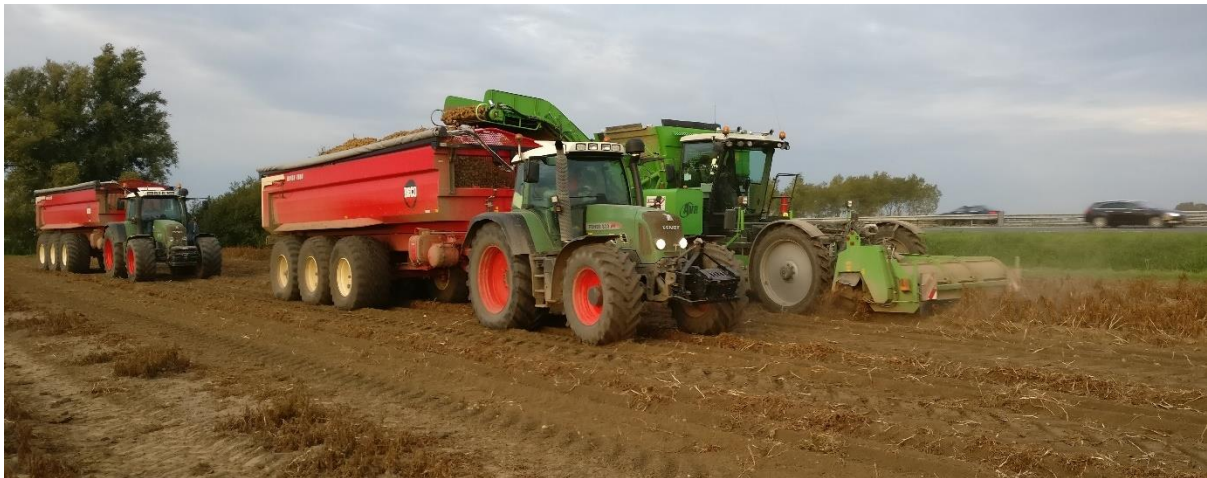
Figure 1: A primary unit (right) harvesting and unloading onto the service unit (left). A second service unit (background) is waiting idle to take over the unit in the centre.
