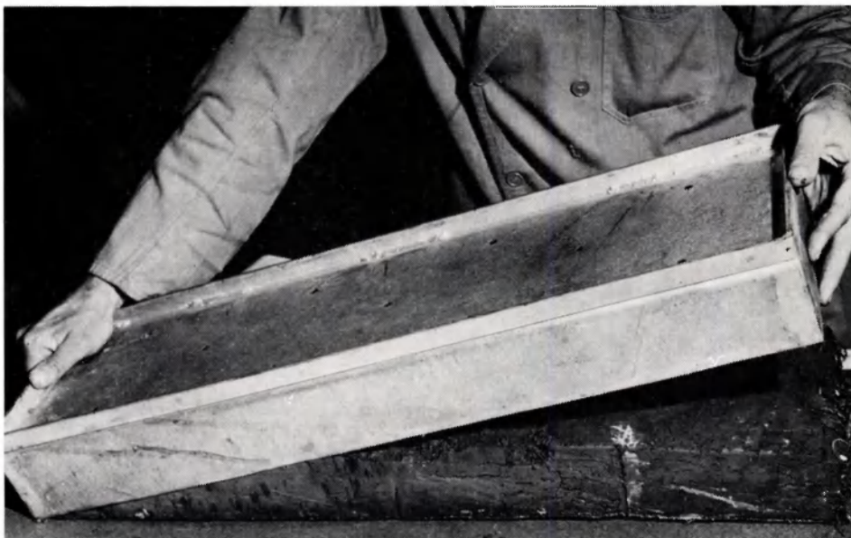
Fig. 21. The box is lifted off the monolith that rests on a piece of hardboard
