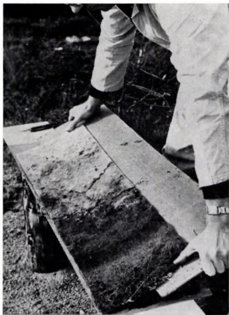
Fig. 9. Transferring the monolith to the prepared piece of particle board
