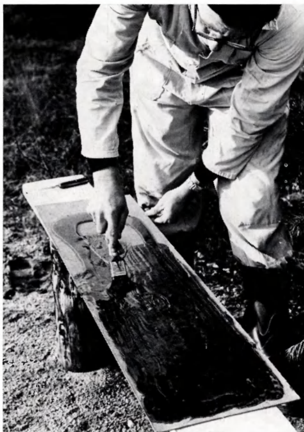
Fig. 8. Applying nitro-cellulose lacquer onto the piece of particleboard
