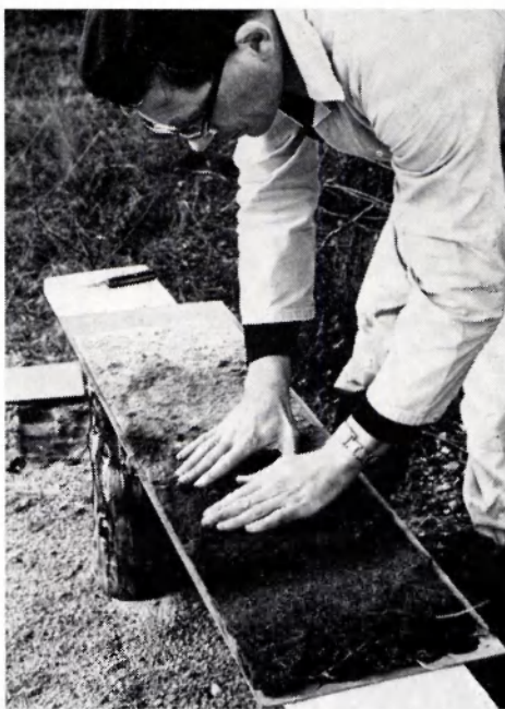
Fig. 10. The monolith is gently pressed down with the flat of the hand
