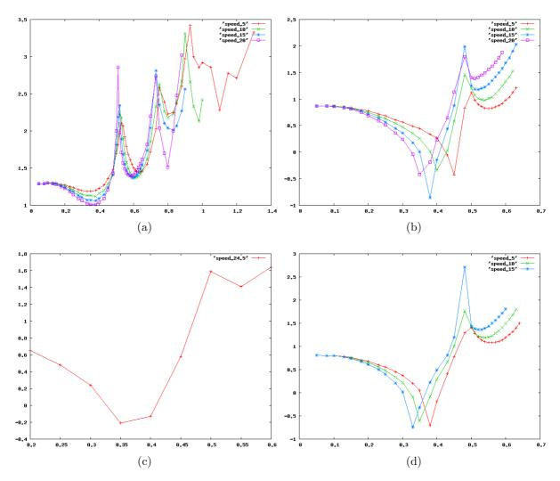
Figure 1.5: Logarithm of threshold amplitudes  $\alpha$  of a single frequency wave forcing as a function of the wave frequency  $\omega$  for different speeds of the vessel. (a) Vessel X for a large range of wave frequencies. (b) Vessel X for low frequency waves in more detail; note the low threshold value at  $\omega = 0.4$ . (c) For vessel Y a similar, but less pronounced, resonance is found. (d) Result for vessel Z.
