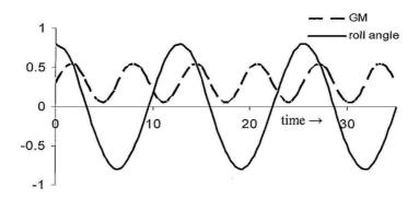
Figure 1.2: Roll angle in the course of time in the resonant state. Note that the period is twice the period of the wave. The dotted line denotes the variation of the metracentric height GM from the waves.
