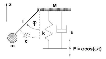
Figure 1.4: Driven spring-pendulum model for heave-roll motion.
