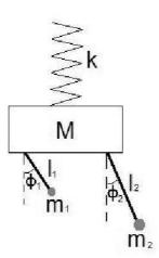
Figure 1.6: Spring and two-pendulum model for heave-roll-pitch motion. Note that in this model there is no direct interaction between roll and pitch.
