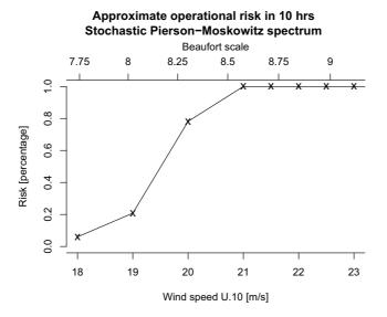
Figure 1.10: Risk of parametric roll (angle larger than 20 degrees) for waves having a Pierson-Moskowitz spectrum at different wind speeds.
