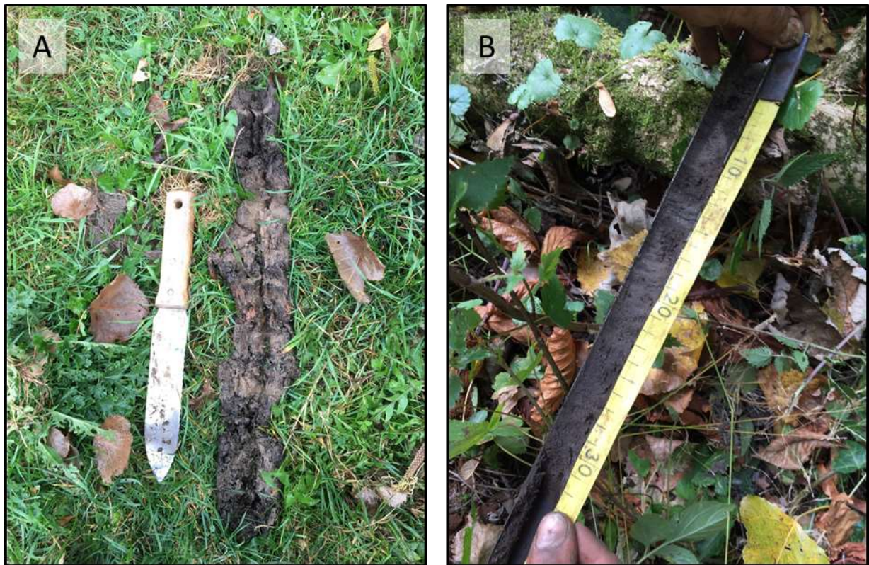
Figure 10. Organic layering in the subsoil. A. Clear layering from 80 cm and onward on the outer bank of the Chaamse Beek, taken with a van der Staay suction corer. B. Slightly distinguishable organic layering from 90-120 cm on the inner bank of the Reusel + Raamsloop stream, taken with a gouge.
