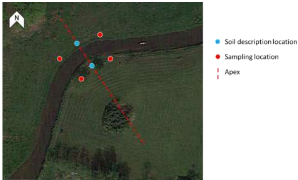
Figure 6. Sampling locations for texture measurements; example is from the Dommel.
