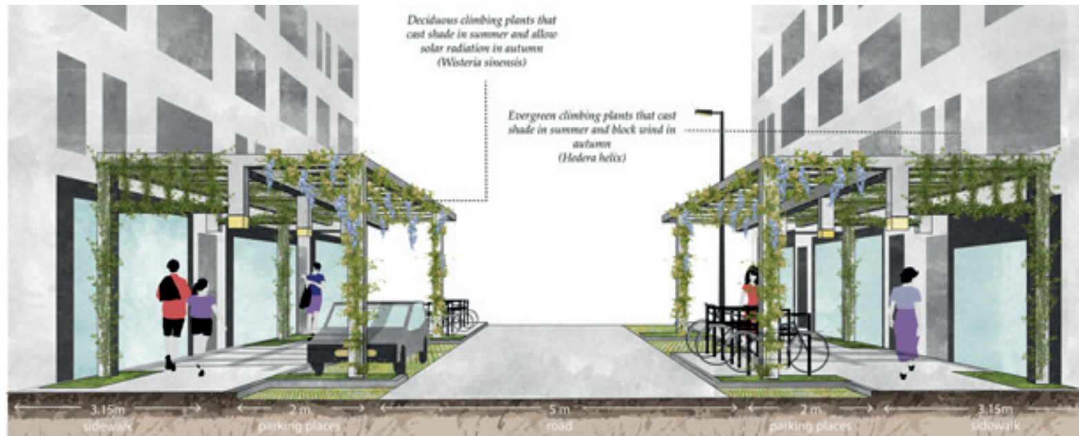
Figure 6.6.8 Semi-evergreen berceaus above parking implemented in the Hoogstraat
