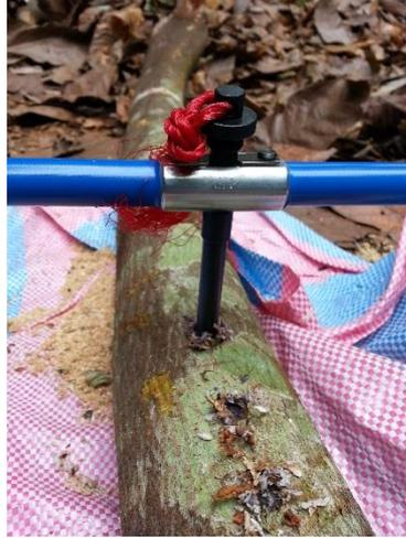
Figure 7. Use of increment borer
