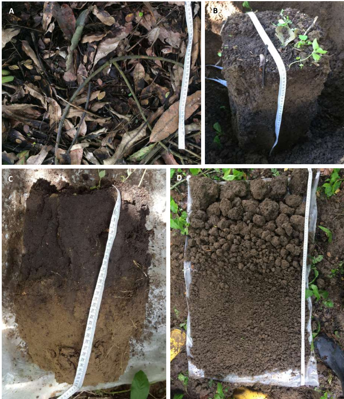
Figure 18. Visual soil analysis sampling process. A. Assessment of percentage of soil cover. B. Excavation of soil block. C. Extraction and placement of soil block over a plastic sheet. D. Ordering of aggregates by size.
