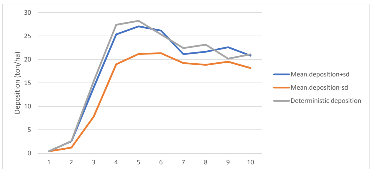
Figure A. 33 Deposition and standard deviation for DEMs with resolution of 2.5 m, 1st type of error for HCL-scenario
