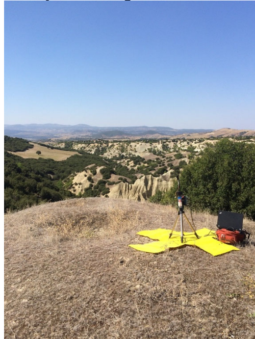
Figure 4 Measuring the GCP coordinates and height with a Rover.
