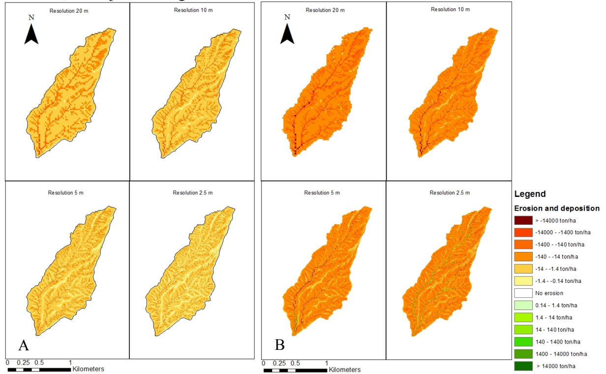
Figure 27 with A - Net erosion maps over 10 years of simulation for the L scenario based on the deterministic DEM, B - Net erosion maps over 10 years of simulation for the H scenario based on the deterministic DEM
