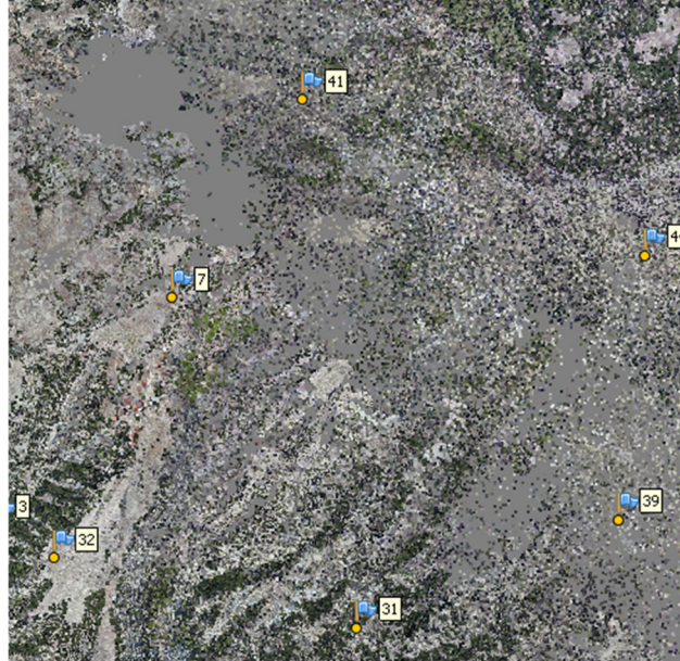
Figure 10 Point cloud, north-eastern part of the study area, grey colour shows the gaps in the point cloud.
