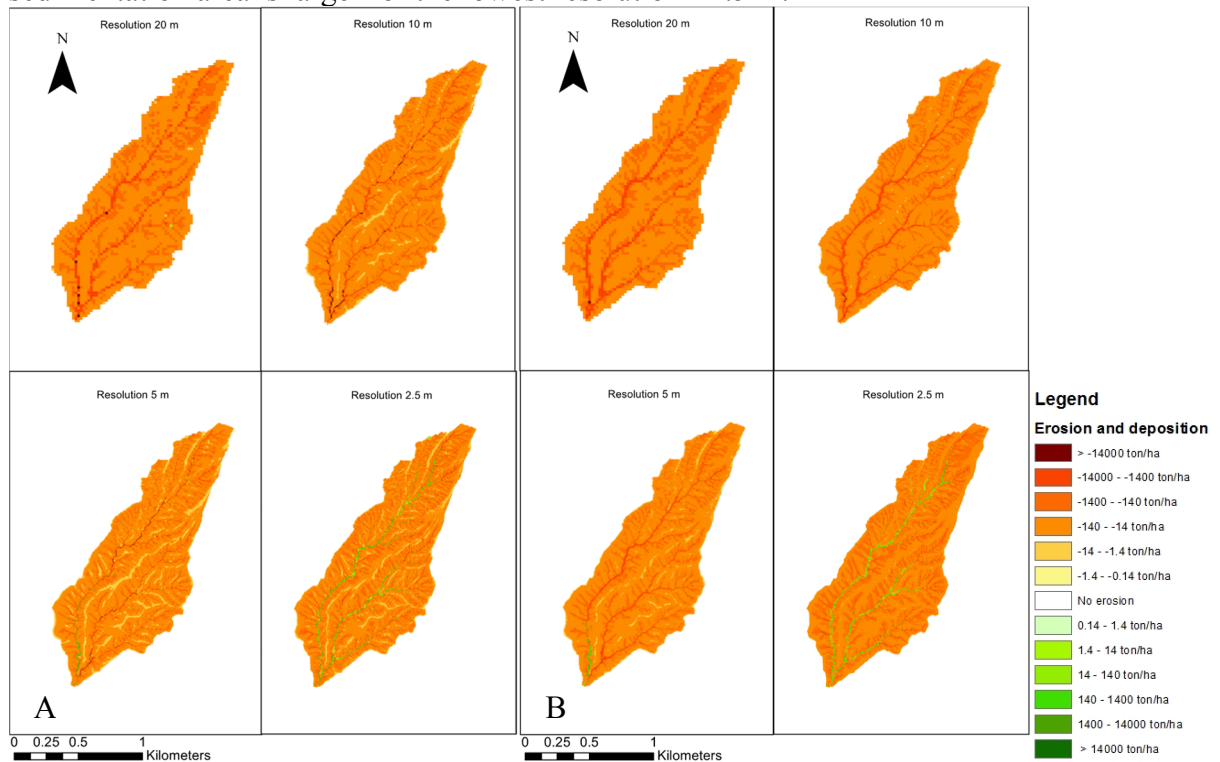
Figure 26 with A - Maps of mean net erosion for the 10 years of simulation for the H scenario with first type error, B - Maps of mean net erosion for the 10 years of simulation for the H scenario with second type error
