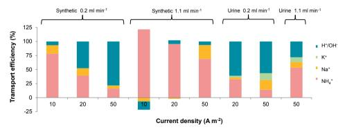
**Figure S3.1.** Transport efficiency of  $NH_4^+$ ,  $Na^+$ ,  $K^+$  and  $H^+/OH^-$  over the membrane. Negative numbers mean transport from cathode to anode, and efficiencies higher than 100% indicate diffusion.  $Mg^{2+}$  and  $Ca^{2+}$  were not detected and therefore did not contribute the charge transport.
