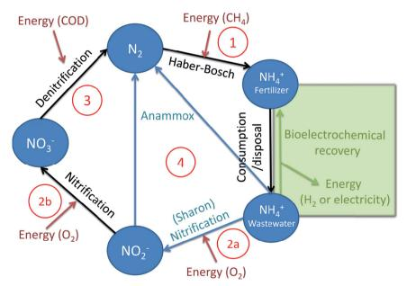
Figure 2.1. The nitrogen cycle in fertilizer production and wastewater treatment processes.
