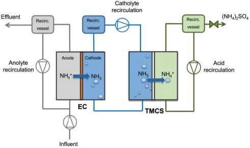
**Figure 3.1.** Schematic representation of experimental setup. EC= Electrochemical Cell; TMCS= TransMembrane ChemiSorption. There were two membranes in the system: a cation exchange membrane in the EC and a gas-permeable hydrophobic membrane in the TMCS unit.
