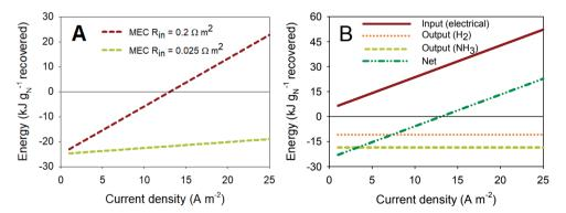
**Figure 2.5 (A)** Energy recovery in an MEC as a function of current density for high (200 m $\Omega$  m<sup>2</sup>) and low (25 m $\Omega$  m<sup>2</sup>) internal resistance. The energy recovery for an MFC is not shown since it is comparable to the MEC. Figure 2.5 **(B)** shows a more detailed overview of the energy input (electrical) and output (hydrogen and ammonia) for the MEC with an internal resistance of 200 m $\Omega$  m<sup>2</sup> as a function of current density.
