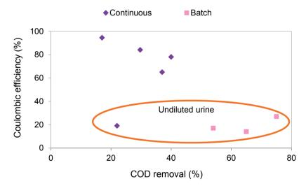
**Figure 6.2**. Coulombic efficiency versus COD removal from different BES studies for the recovery of TAN from urine (data from Table 6.3, taking the average of our data with undiluted urine)
