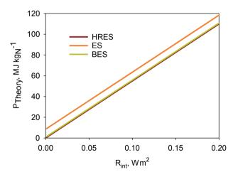
Figure S4.2. Theoretical power demand evaluated as a function of the internal resistances.
