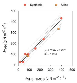
**Figure 3.2.** TAN flux over the cation exchange membrane  $(J_{TAN})$  against NH<sub>3</sub> flux over the TMCS membrane  $(J_{NH3, TMCS})$ . The regression line was fitted only for the synthetic wastewater points for modelling purposes. Long-dashed and short-dashed curves represent the 95% confidence interval and 95% prediction interval for the linear regression, respectively. This figure shows that the system was near steady state.
