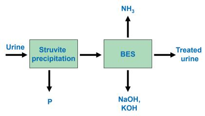
Figure 2.3. Proposed full treatment concept for urine, in which ammonium is recovered using a BES
