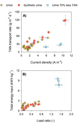
**Figure 5.3 A)** TAN transport rate with respect to current density and **B)** total energy input with respect to load ratio from a bioelectrochemical system treating real and synthetic urine at different dilutions and urine with 70% less TAN (urine was pre-treated with a TMCS).
