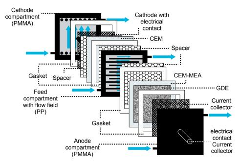
Figure S4.1. Schematic representation of the HRES cell design and its components.
