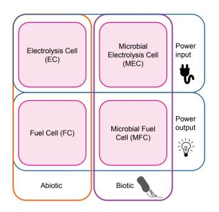
**Figure 1.4.** Classification of (bio)electrochemical systems used for the recovery of TAN (based on [62]).
