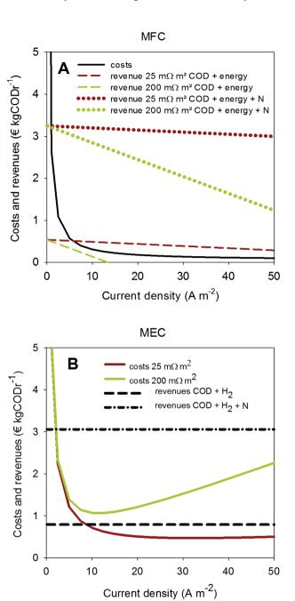
**Figure 2.6.** Comparison of the costs and revenues of ammonia recovery in an MFC **(A)** and in an MEC **(B)**. The costs and revenues are shown at different internal resistances of the system and with and without the recovery of ammonia
