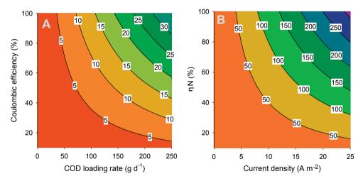
**Figure 2.4.** (A) Current density (A m<sup>-2</sup>) as a function of the coulombic efficiency (%) and the loading rate (g d<sup>-1</sup>) and (B) ammonium flux from anode to cathode (g d<sup>-1</sup>) as a function of transport efficiency (%) and current density (A m<sup>-2</sup>).
