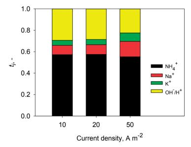
**Figure 4.3.** Contribution of ionic species to the total charge transport through the CEM. Ammonium ions were the main charge carrier in all experiments independent of the current density.
