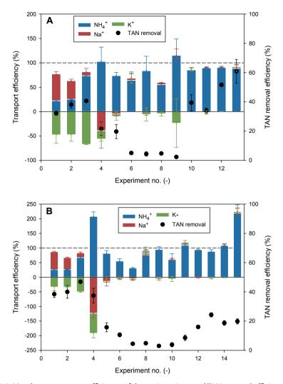
**Figure S5.2**. Membrane transport efficiency of the main cations and TAN removal efficiency for each experiment performed in **A**) Run 2, and **B**) Run 3
