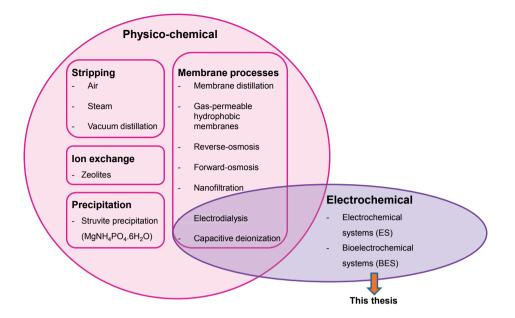
**Figure 1.2.** Different techniques for the recovery of TAN from nitrogen-rich wastewater streams (based on [38, 51]). The recovery by nitrogen incorporation into biomass (such as microalgae cultivation) has been excluded in this overview. This thesis involves the use of electrochemical and bioelectrochemical systems.
