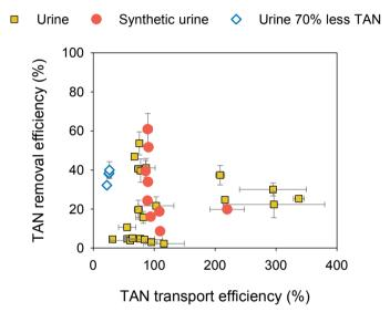
**Figure 5.2.** TAN removal efficiency with respect to transport efficiency from a bioelectrochemical system treating real and synthetic urine at different dilutions and urine with 70% less TAN (pretreated with a TMCS).
