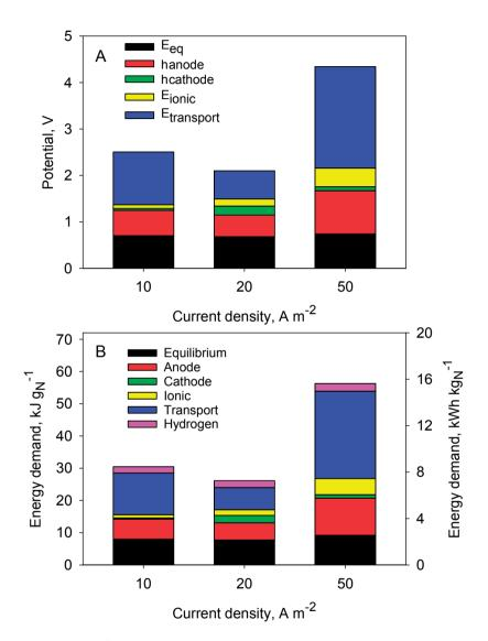
**Figure 4.2. (A)** Analysis of the internal voltage losses and **(B)** energy demand determined during the experiments at different current densities. Equilibrium voltage  $(E_{eq})$ , anode overpotential and transport losses over the CEM (between feed and cathode compartments) are the main source of potential in all experiments. The additional H<sub>2</sub> (about 10%) supplied by the electrolyser account for only 4 to 9 % of the energy demand.
