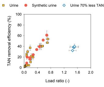
**Figure 5.1.** TAN removal efficiency with respect to load ratio from a bioelectrochemical system treating real and synthetic urine at different dilutions, and urine with 70% less TAN (pre-treated with a TMCS).
