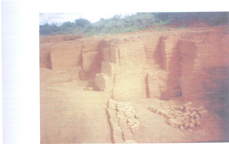
Plate 6. Active plinthite mine on upland soil at Hounde in Burkina Faso. The plinthic layer is over 20 m thick.
