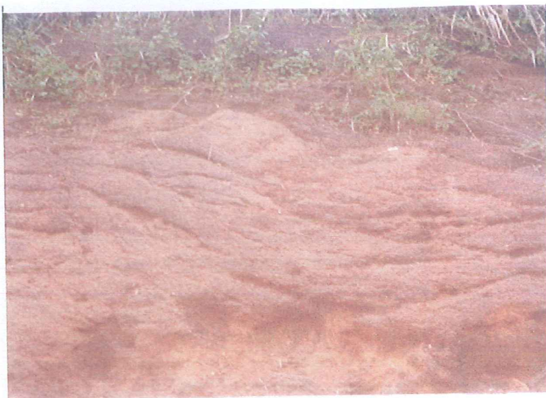
Plate 8. Petroplinthite formed on the surface of a road cut through upland soils near Duayaw Nkwanta (Brong Ahafo Region)
