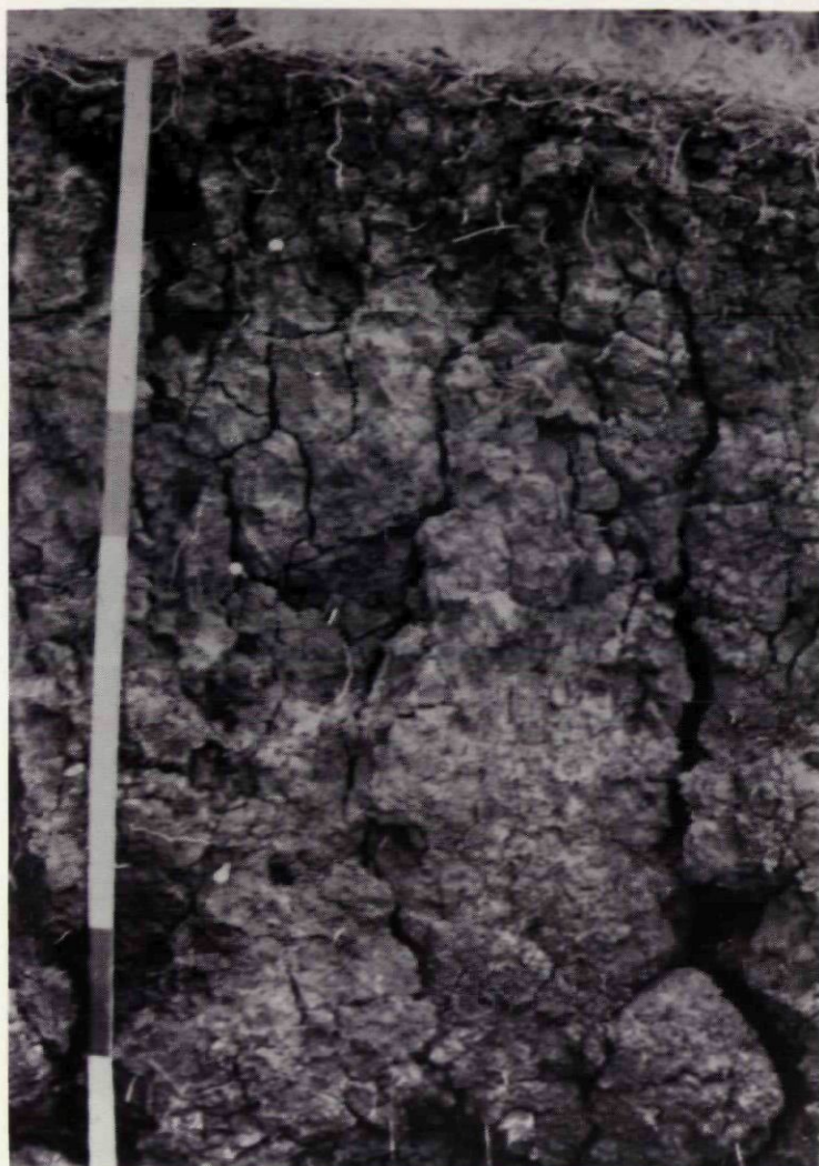
Fig. 8.5 Soils of mapping unit PIA2 consist of cracking heavy clay of lacustrine origin.
