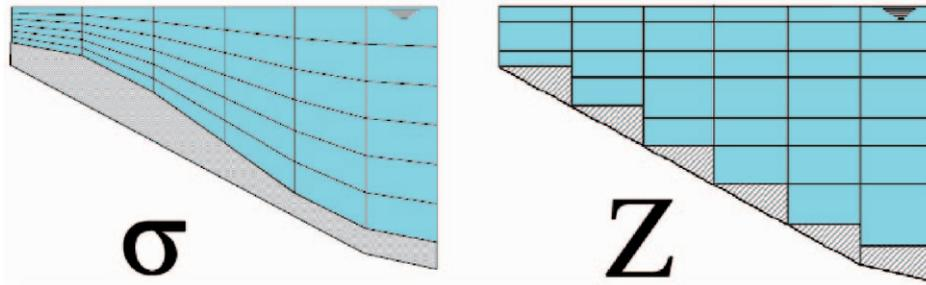
FIGURE 4.2 HYDRODYNAMIC GRID SCHEMATISATION FOR (A) DELFTSE HOUT AND (B) GOOIMEER-EEMMEER
