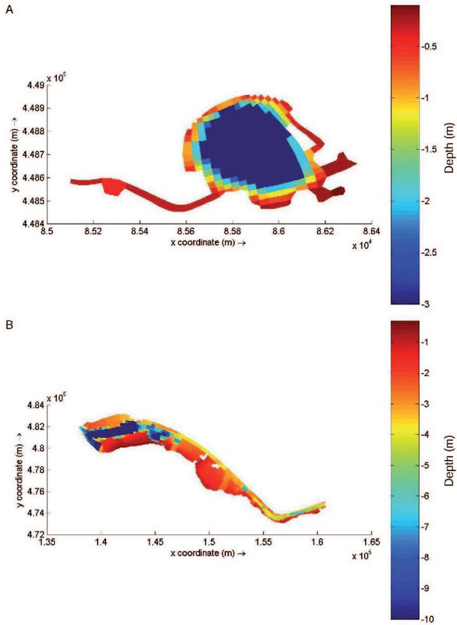
FIGURE 4.5 HYDRODYNAMIC MODEL BATHYMETRY FOR (A) SLOTERPLAS AND (B) WESTEINDERPLASSEN
