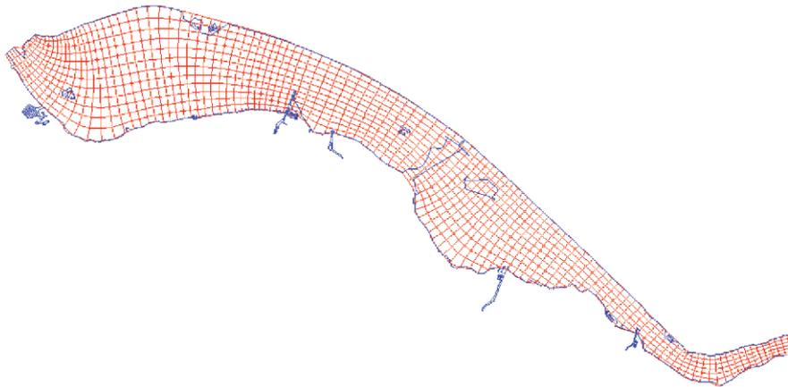
FIGURE 4.3 HYDRODYNAMIC GRID SCHEMATISATION FOR (A) SLOTERPLAS AND (B) WESTEINDERPLASSEN
