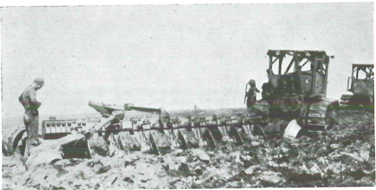
Fig. 3. —A disc-type breaking plow developed by Mr. O. B. Lasiter and used on the Alberta Land Clearing Project. Recent improvements in construction and design have enhanced the value of this type of plow for breaking land in this area.
