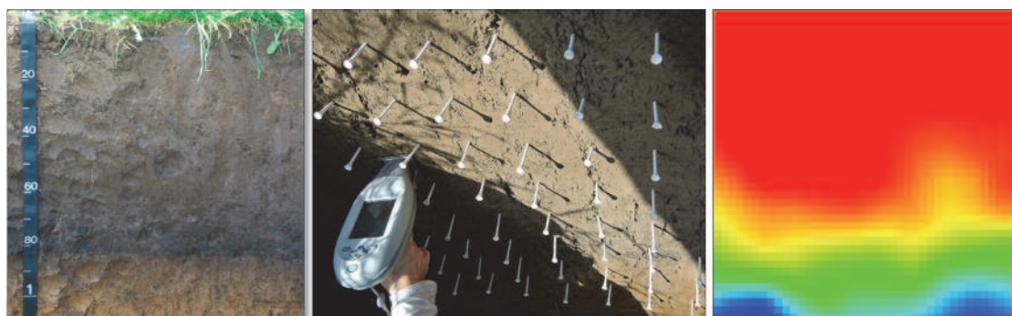
Figure 2. A Mollisol (Phaeozem), hand-held XRF, and a map of the Fe content of the same profile (1 by 1 m, values increase from red, through yellow and green to blue)
